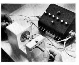
ELECTRICAL CONTACTS of switch can be activated by this special tool for testing. The tool also measures the exact travel distance of the internal piston. After this test, the switch is filled with silicon oil and sealed.
